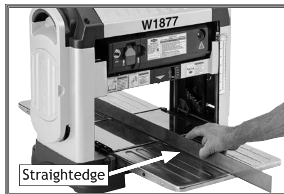
Figure 17. Aligning extension tables.
