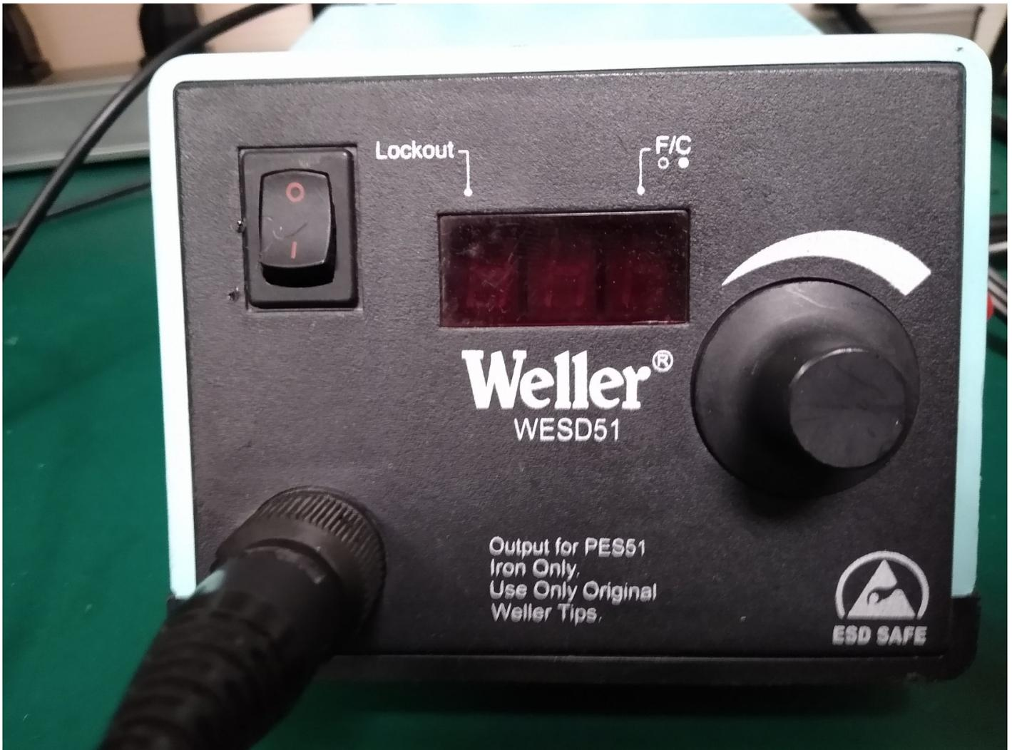
The Weller® PES51 tools are interchangeable without the need to make any adjustments to the station "Offset" function. This is made possible by the use of a precision temperature sensor; which is positioned deep inside the tip to insure rapid response to soldering load variations. The Weller® PES51 tool has been specifically designed for use at electrostatic free workstations and is completely free from stored static charges.
