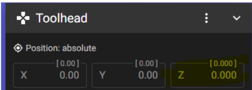
**Move the Nozzle:** Manually move the print head to each corner of the bed using the printer's control panel or software. Ensure that the nozzle is positioned directly above the corner. *Place a Sheet of Paper: Take a sheet of standard printer paper or a thin gauge feeler gauge. Slide it under the nozzle while adjusting the bed height. The paper should have a slight resistance when moving under the nozzle.*
