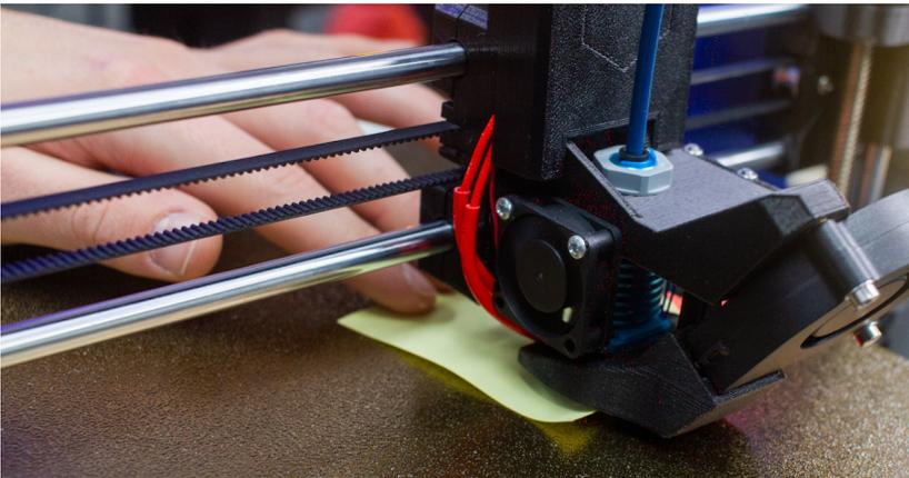
Home the Printer: Start by homing the printer, which will position the nozzle at its starting point.
